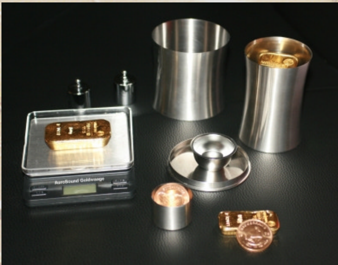
Density determination of gold bars and gold coins with some of the stainless steel measuring cups of the testing set ATS 1000
